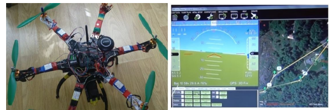
Figure 8: The hexacopter with APM 2.6 flight controllers and its flight by telemetry
