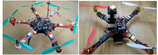
Figure 7: Photo of the hexacopter and quadcopter with an ATmega2560 Based Flight Controller
