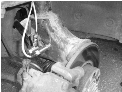
Fig.1. Front wheel support with installed VIB and SPM transducers
