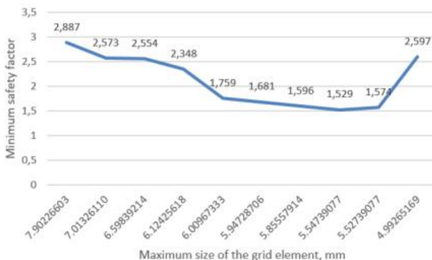
Fig. 3. Dependence of the minimum safety factor on the maximum size of the grid element
