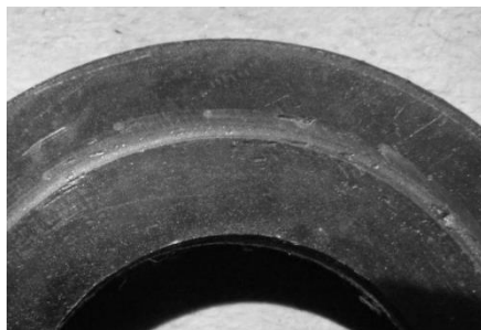
Friction track of a sample made of 40X steel, tempered and nitrided 183 hours of work
