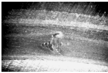
Friction track of a sample made of 40X steel, tempered and nitrided 183 hours of work
