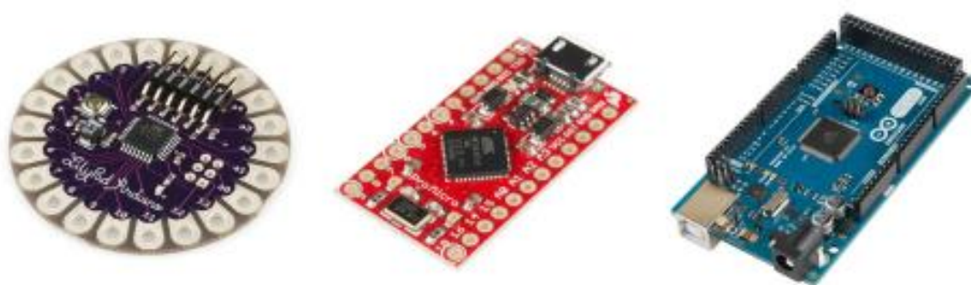
(From left to right) Lilypad, Sparkfun Pro Micro, Arduino Mega
