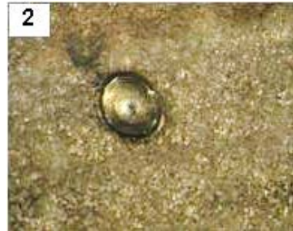
Fig. 3. Stereoscopic photograph of a Cu-Mo coating laser-eroded at 20 W (x57 magnification)
