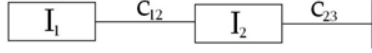
Fig. 2. Calculation scheme of the main line of the plug-mill: I – inertia moment of working shafts; I – inertia moment of pinion stand; c_{12} – rigidity of spindlessection of transmission; c_{23} – rigidity of interval shaft of transmission
