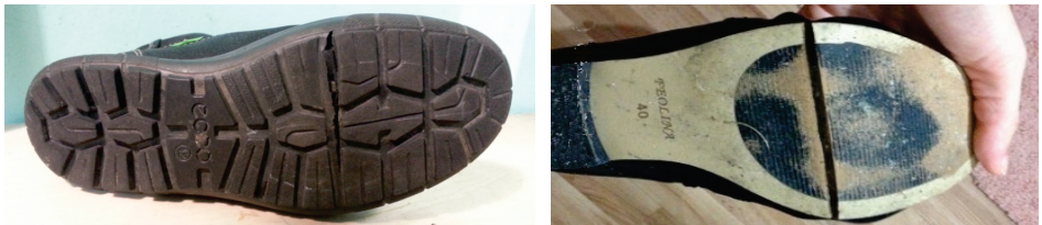
Fig. 1.17. Destruction of double-shoe polymer parts of shoes when bending [own study]
