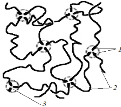
Fig. 2.1. Schematic structure of butadiene styrene thermo elastic plastic: 1 – polystyrene blocks; 2 – butadiene blocks; 3 – polystyrene domains [own study]
