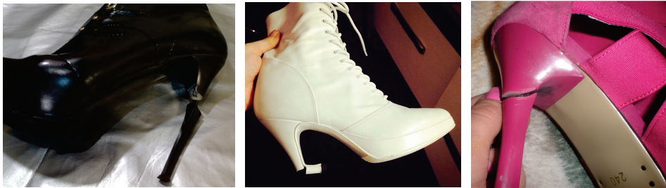
Fig. 1.16. The destruction of the cantilevered shoe parts at their bend [own study]
