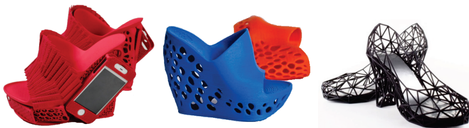
Fig. 1.12. Polymeric footwear created using 3D printing technology [48]
