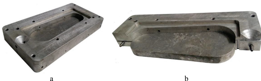
Fig. 4.10. Mold for soles with particles of recycled waste addition: a – semi-closed state; b – closed state [own study]
