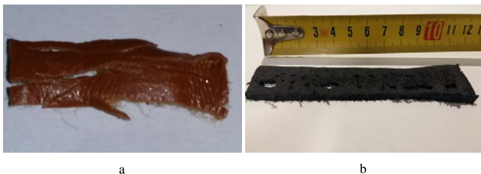
Fig. 3.40. Formation of the free surface of the polymeric specimen: a – polypropylene artificial leather; b – PVC sole [own study]
