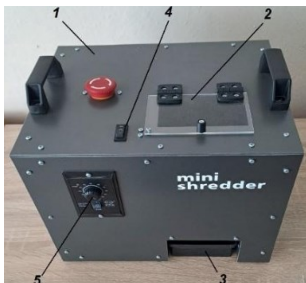
Fig. 2. Mini-shredder for shredding polymer waste: 1 – frame; 2 - loading hopper; 3 – container for collecting shredded material; 4 – switch; 5 – cutting shaft speed regulator
