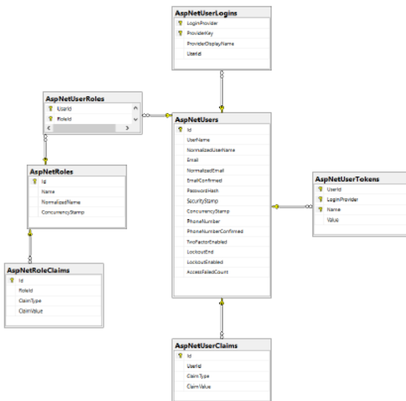
Figure 2. Datalogic model of the website database
