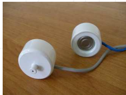
Fig. 27. Constructive realization of the block of the microcontroller and sensor of surplus pressure on the basis of PRMT
