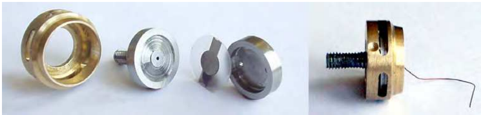
Fig. 22. Elements and construction of PRMT with PM
