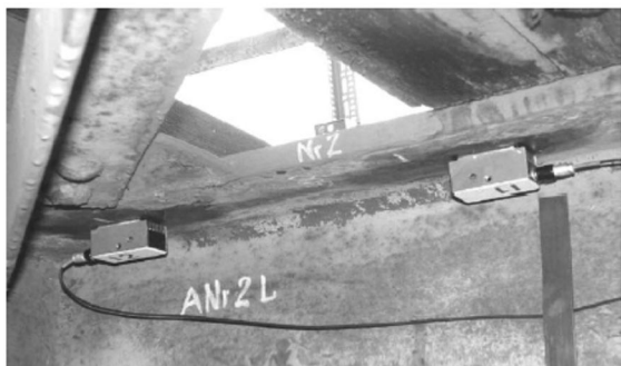
Fig. 7. The head of IMPUL system of the lower surface of the upper shelf beam
