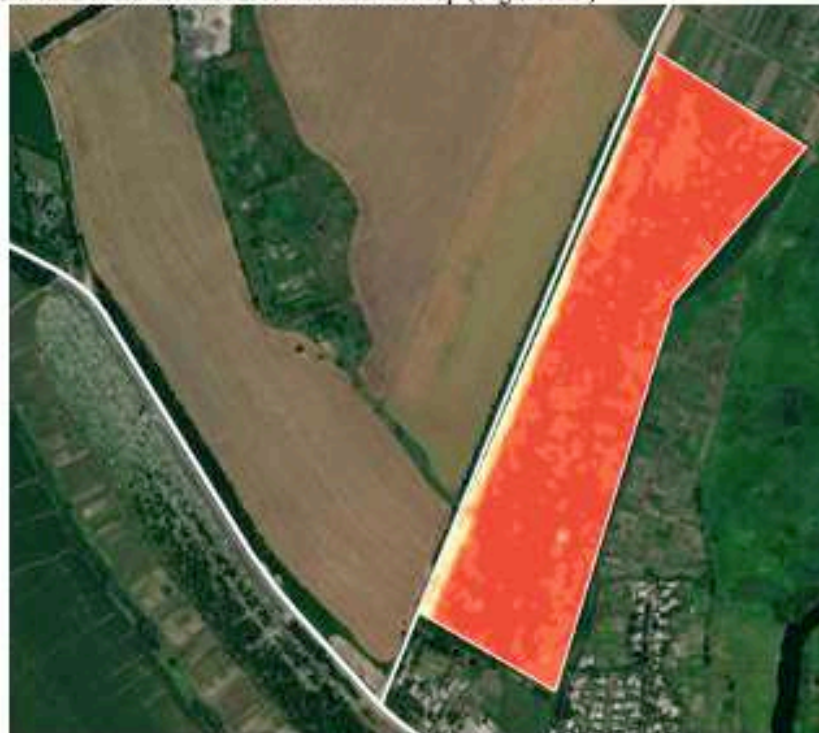
Figure 1.9 - Resource Allocation Map (GIS Map with Variable Rate Application Zones)
