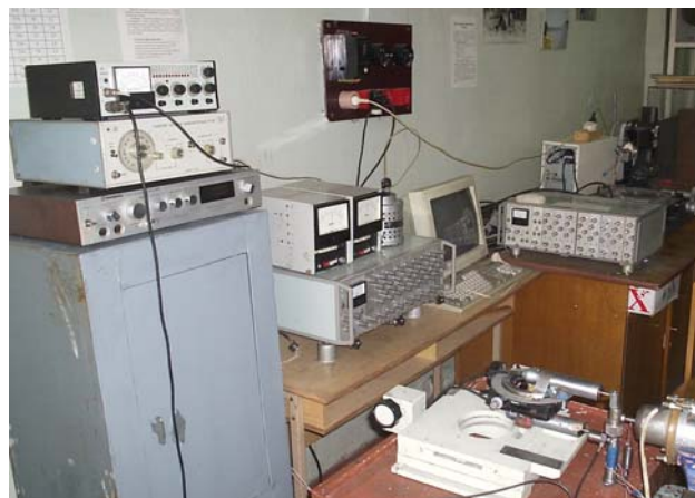
Fig. 2. The plant for a research of frictional contact in conditions fretting.
