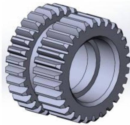
Fig. 2. Solid-state model of the gear blockper
