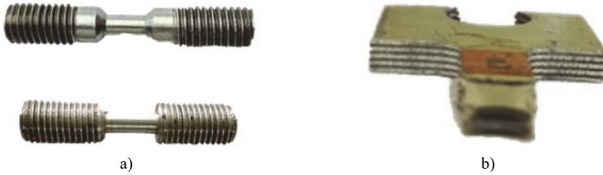
Fig. 1. Samples for testing: a) cylindrical specimens; b) a flat multilayered specimen after failure
