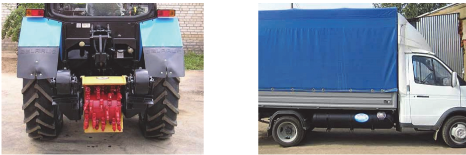
Fig. 21. General view of a road mill and vehicle with cylindrical balloon for gas
