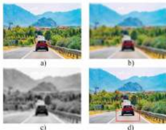
Fig. 4. Stages of car recognition in a photo: a) Reading a frame from a video stream b) Image blurring and noise reduction c) Converting the image to black and white d) Detected car
