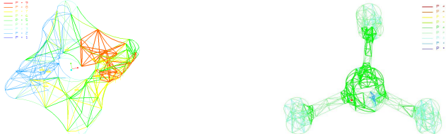
Fig. 7. Mesh adaptation of models using p-elements
