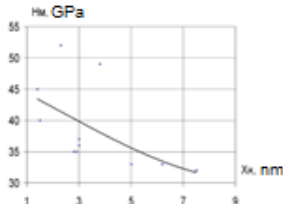
Fig. 2. Microhardness of the coating, depending on the crystal size
