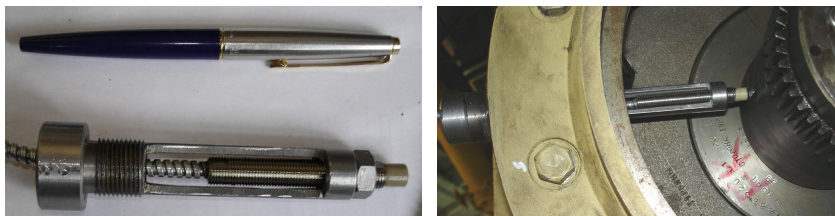
Fig. 2 The proximity probe in custom design housing for internal-external mounting (KTU Mechatronic Science Laboratory courtesy)
