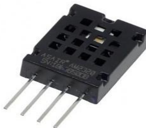
Figure 2.4– Temperature and humidity sensor AM2320
