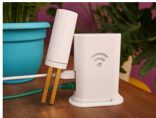
Figure 1.11 – The Plant Link Wireless Plant Sensor
